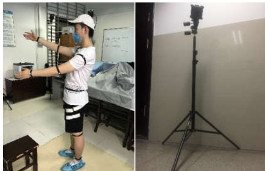
Fig.2 Subject wearing the motion capture device (left) and the motion recording equipment Cortex (right)
