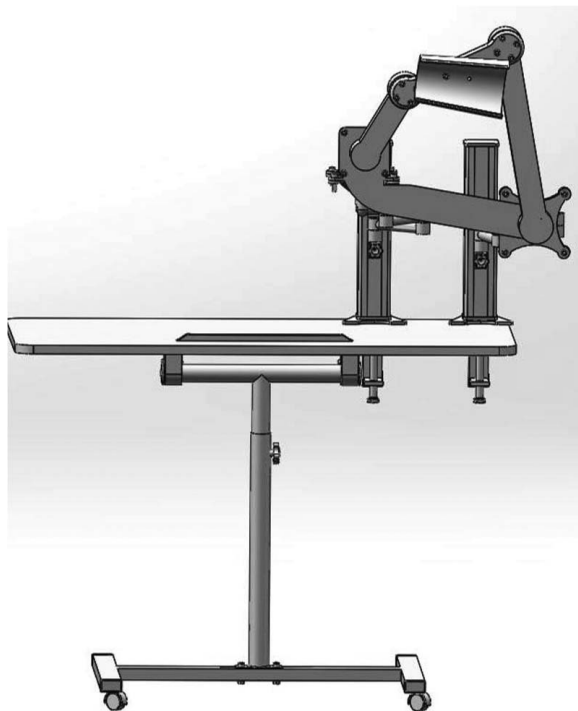
Fig. 6 Design of the upper-limb rehab device incorporated with the one-DOF motion executor as shown in Fig. 5
